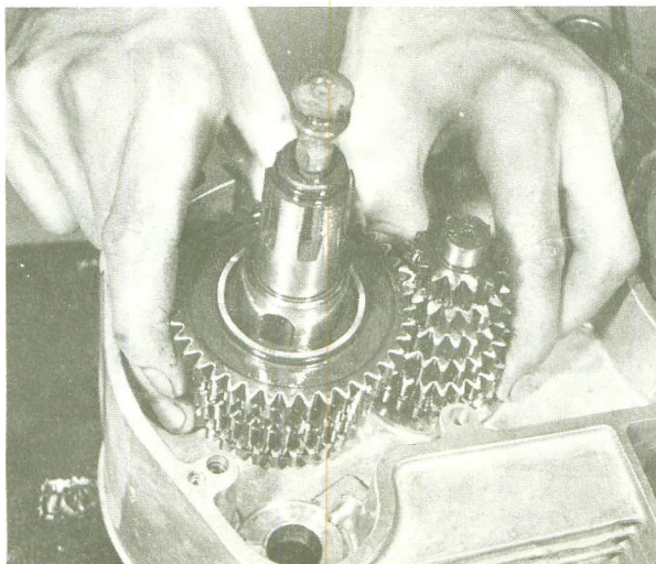
59.2 Replace the gears in the crankcase
